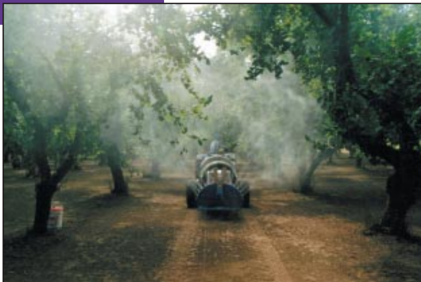
Electrostatic sprayers are used to apply crop protectants to hazelnut orchards.
